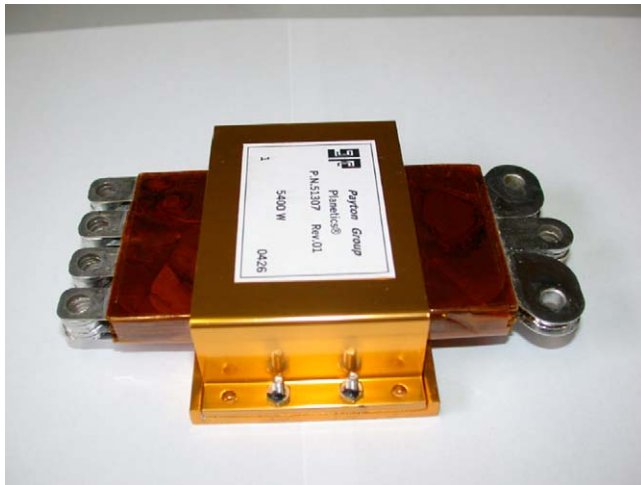
Fig. 6. 5400 W–50 kHz PAYTON planar transformer.
